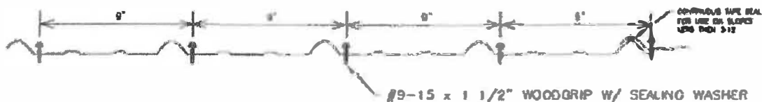
FASTENER PATTERN AT 24" O.C.
